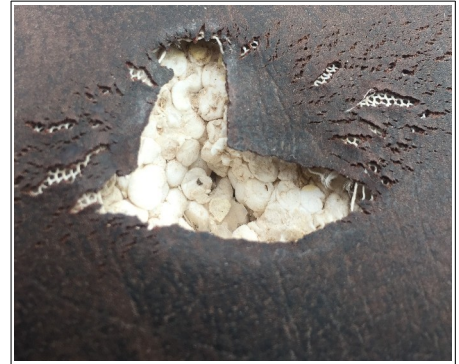
The hole in this vinyl must be subpatched before applying filler.
